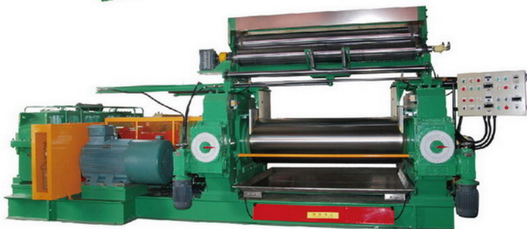
26"x84" (雙馬達、雙進雙出型) Twin motors, Twin output shafts.
