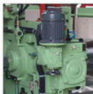
電動調整 (選配) Motor power-zoom (optional) 方便調整兩輪間距 It's more easy to modify the gap of two rollers.
